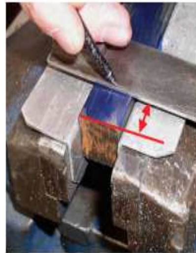
Use a rule, scribe and square to mark the hole positions along the centerline working from the datum at one end of the bar.
