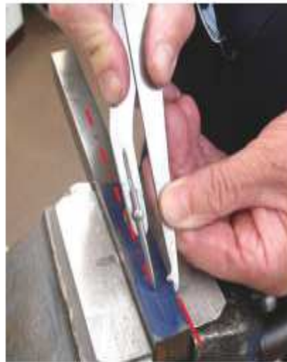
Use odd-leg calipers to find and scribe the centerline along the bar using one edge as the datum.
