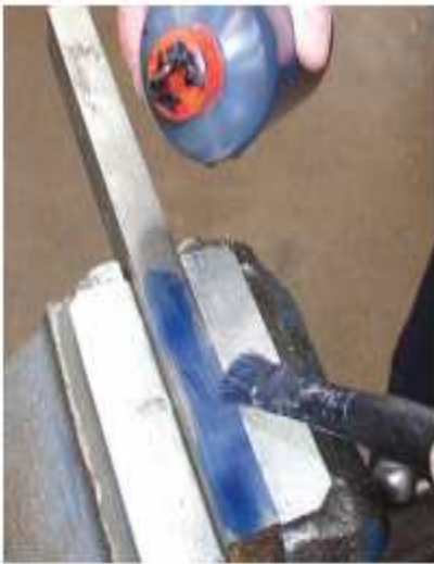
Brush a thin layer of marking blue onto the surface of the metal bar to highlight the lines.
