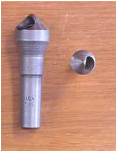
Side and end view of a cross-hole deburrer
