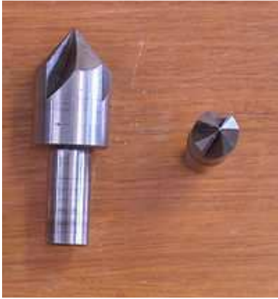
Side and end view of a 4 fluted countersink
